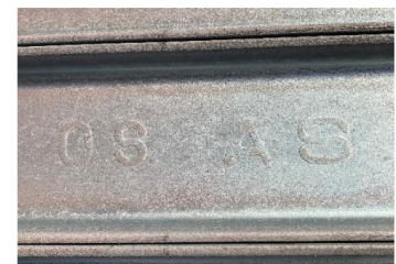
TAPERED FLANGE BEAM
